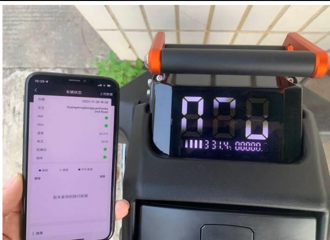
1 Battery voltage check
