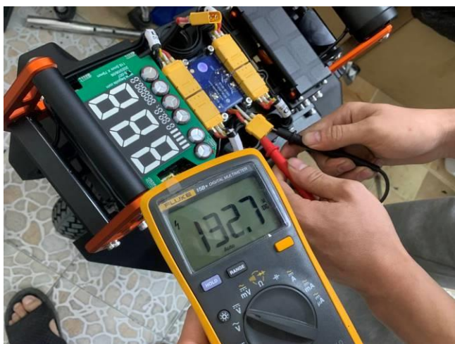
Battery voltage check
