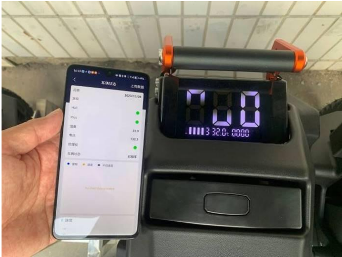
3 Battery voltage check
