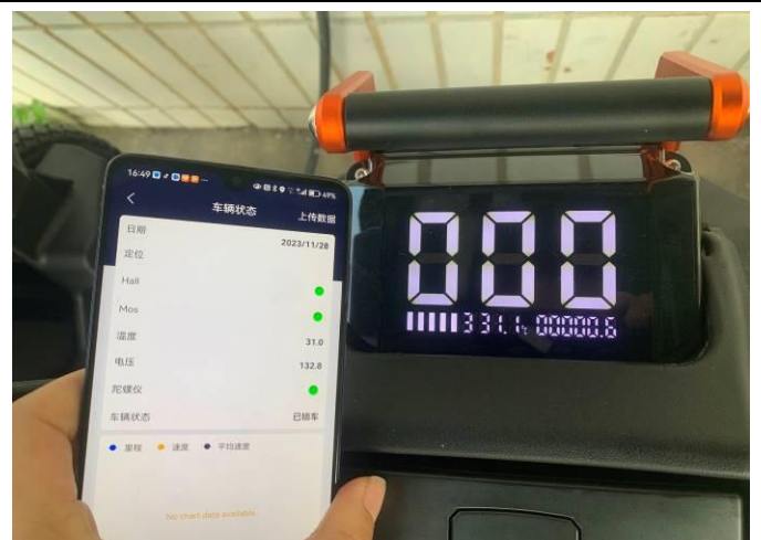
2 Battery voltage check
