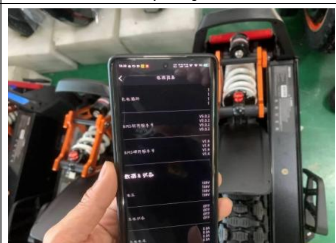
12 Battery voltage check
