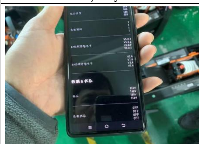
13 Battery voltage check
