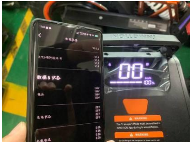
Battery voltage check By App:
