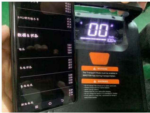
Battery voltage check By App:
