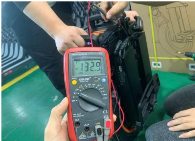
23 Battery voltage check
