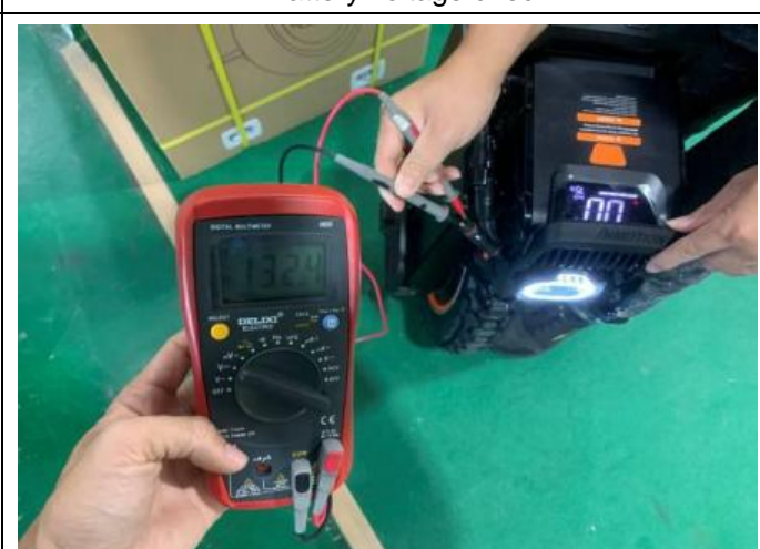
14 Battery voltage check
