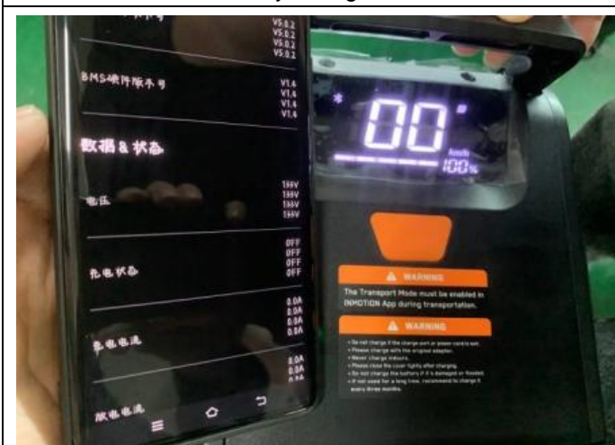
11 Battery voltage check
