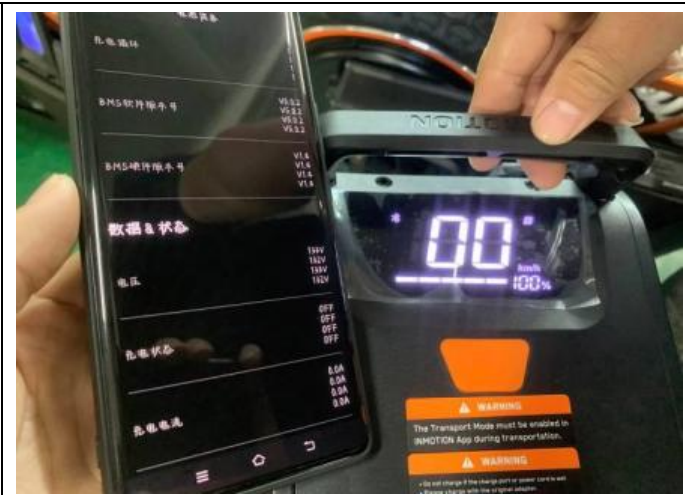
10 Battery voltage check
