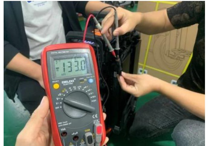
18 Battery voltage check
