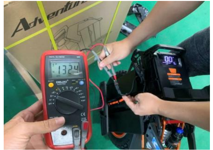
16 Battery voltage check
