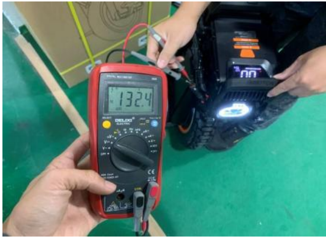
15 Battery voltage check
