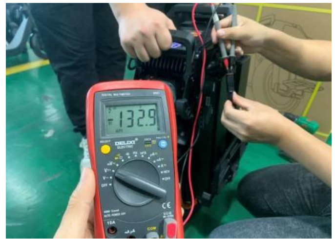
22 Battery voltage check
