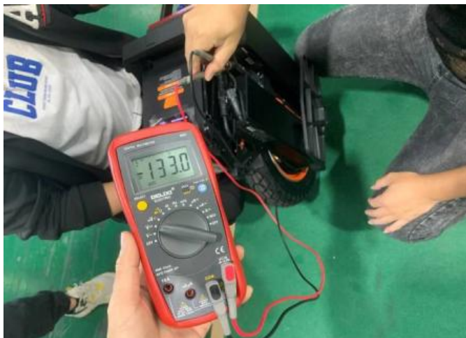
19 Battery voltage check
