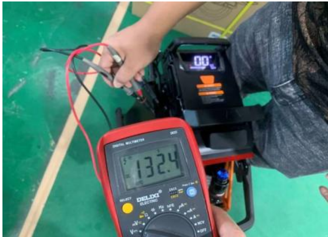
17 Battery voltage check
